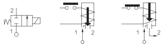
Max allowable pressure (PS) 16 bar - According to EN 60730-2-8 - Factor of safety for domestic applications equal to 5 times PS
